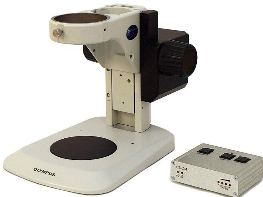
PRO-SZM1 motorized focus drive on SZ2-ST stand with CB-ZM control unit
