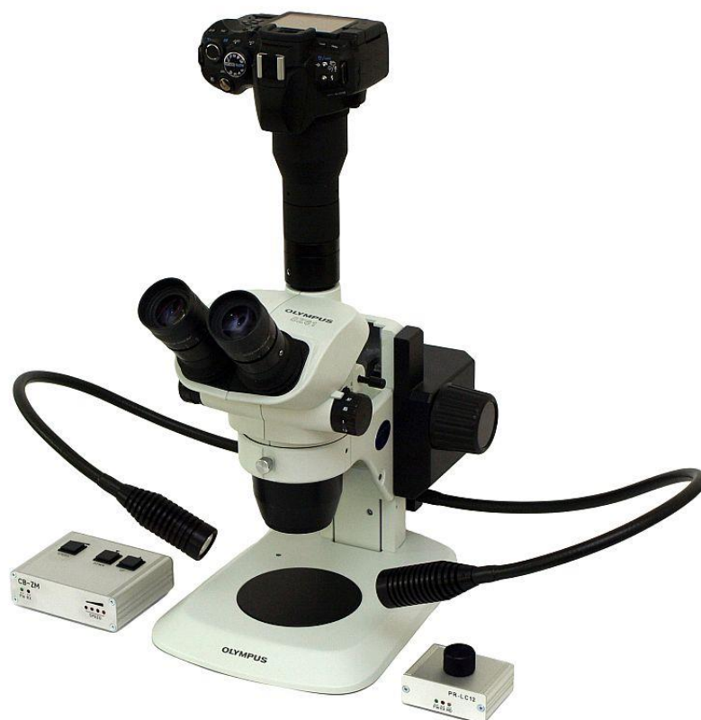
Motorization of OLYMPUS® SZ61 stereomicroscope
