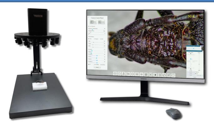
PRO-18 AF 4K device with optional illuminator for large samples and 28" 4K UHD monitor
